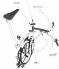
Stage 2: Unfold handlebars and do up handlebar clamp (HCPL)
