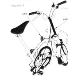
Stage 3: Standing behind the bike, right hand on saddle, left hand on handlebar stem (HBS); rock the saddle back slightly and unhook the front wheel from the rear frame. Then, using a stirring motion, bring the front wheel to the front of the bike. Do up the main frame clamp (MH)
