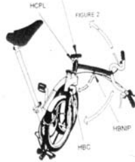
Stage 2: Unfold handlebars and do up handlebar clamp (HCPL)
